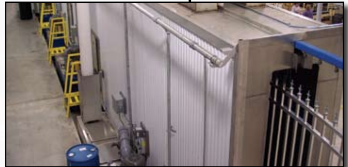
The next four stages consist of a: STEP #3: (CLEAN) City water rinse, STEP #4: (CLEANER) Recycling reverse osmosis water rinse, STEP #5: (CLEANEST) Pure reverse osmosis water rinse, and STEP #6: Primer/sealer conversion coating.
