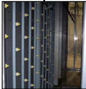
STEP #2: Product enters heated acidic cleaner stage to remove extrusion and fabrication oils.
