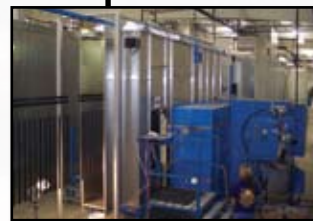
STEP #9: Powder application is automated. Compressed process air is dried to -35°F Dew Point for superior adhesion and aesthetics. The powder booth contains powder coating overspray with no emissions to the surrounding environment.
