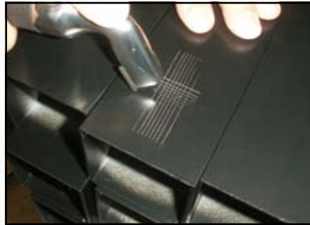
ASTM D3359 Crosshatch Test Hourly crosshatch testing is completed per ASTM D3359 to test coating adhesion.
