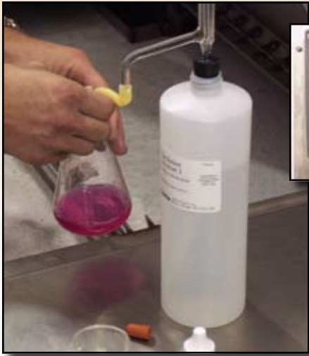
Automated Chemical Test Pretreatment chemicals are monitored and added automatically but titration is checked manually twice per shift.
