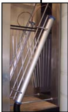
STEP #7: A 200 MPH air blast removes water drops from the pre-treated product.
