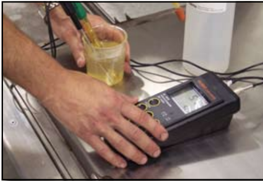
System Titration Test Ph levels are checked twice per shift as part of the pretreatment titration check.
