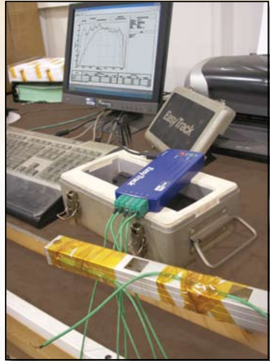
Cure Oven Temperature Test Cure oven air temperatures and part temperatures, during the cure process, are monitored frequently to ensure proper curing of powder coating.
